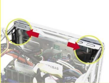
When you start to take the Front Panel apart, please pay attention to the rib that is located at top of the both side panel. As the left picture shown, the first you can pull it apart toward the both side, then softly pull it away. Finally you can pull the Front Panel apart. Be careful not to break the rib.
