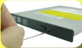
Eject the disc tray by poking the enclosed thin stick into the eject hole.
